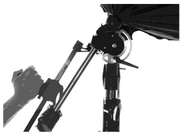
**Extra** force could be needed to open the reflector. Use the special hand clamp that is delivered with the reflector.
