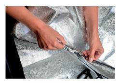
Position the rounded rod end into the loops.
